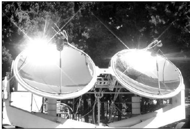
Figure 2. Solar plant with parabolic concentrator.
